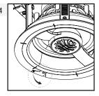
After connecting wires, insert the Speaker into the Bayonet Ring, with the METAL LOCK TAB LIFTED AWAY FROM THE RING.
