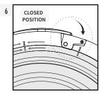
**CLOSED POSITION:** To finalize the installation, **PUSH THE METAL LOCK TAB TOWARDS** the Bayonet Ring.
