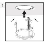
Push the Zip-Clip™ rails inwards, just enough from the top, so they fit through the ceiling hole opening, then INSERT THE BAYONET RING INTO THE CUT-OUT hole within the ceiling surface.
