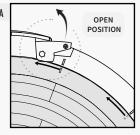
OPEN POSITION: PULL THE METAL LOCK TAB AWAY from the Bayonet Ring, before removing loudspeaker from Bayonet Ring.
