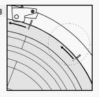
With one hand on the ring & one hand on the speaker, **ONE QUARTER TURN COUNTER-CLOCKWISE** will release the Speaker from the Bayonet Ring.
