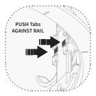
**Note:** If the Bayonet Zip-Clips<sup>™</sup> need to be adjusted or removed, depress the metal tabs along the rail and push up.
