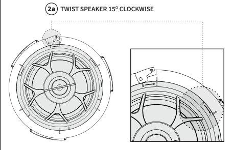
**2b)** When the Speaker is correctly installed into the Bayonet Ring, **THE SPEAK- ER GROOVE LINES WILL BE ALIGNED TO THE MATCHING GROOVE LINES OF THE BAYONET RING.** Then you will be able to move the Ring-Lock Tab inwards, towards the center of the speaker.
