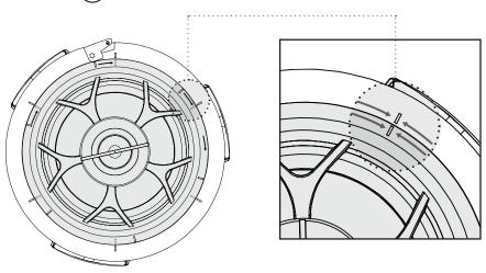
3) LOCK THE SPEAKER INTO THE BAYONET RING: PUSH THE METAL RING-LOCK TAB INWARDS, towards the Bayonet Ring, INTO THE CLOSED & LOCKED POSITION. When this Ring-Lock Tab is fully closed, it should lay flush with the perimeter of the Bayonet Ring.
