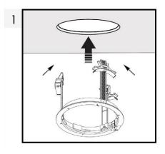
**2)** Reach inside the Bayonet Ring, placing 2 fingers on the grooves of the Bayonet Zip-Clip<sup>™</sup> to pull each Zip-Clip<sup>™</sup> down the rail, until it grips the drywall securely. The Bayonet Ring should be firmly in place, but not too tight.
