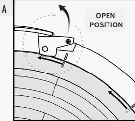
**OPEN POSITION: PULL THE METAL LOCK TAB AWAY** from the Bayonet Ring, before removing loudspeaker from Bayonet Ring.
