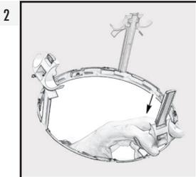
Reach through and **PLACE 2 FINGERS ON THE GROOVES** of the Bayonet Zip-Clip™ to pull each Zip-Clip™ down the rail.
