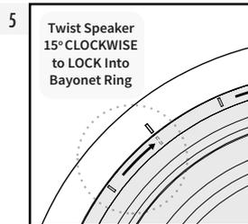
**TWIST THE SPEAKER 15° CLOCKWISE**, until the indicators on both the Bayonet Ring & the Speaker are aligned.
