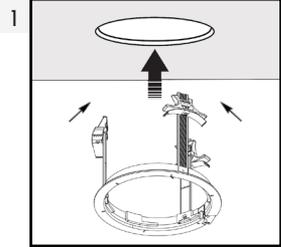
Push the Zip-Clip™ rails inwards, just enough from the top, so they fit through the ceiling hole opening, then **INSERT THE BAYONET RING INTO THE CUT-OUT** hole within the ceiling surface.
