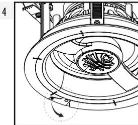
After connecting wires, insert the Speaker into the Bayonet Ring, with the **METAL LOCK TAB LIFTED AWAY FROM THE RING.**
