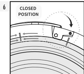
**CLOSED POSITION:** To finalize the installation, **PUSH THE METAL LOCK TAB TOWARDS** the Bayonet Ring.
