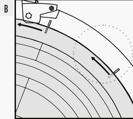
With one hand on the ring & one hand on the speaker, **ONE QUARTER TURN COUNTER-CLOCKWISE** will release the Speaker from the Bayonet Ring.
