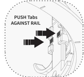
**Note: If the Bayonet Zip-Clips™ need to be adjusted or removed, depress the metal tabs along the rail and push up.**
