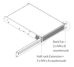
The installation and equipment rack should be configured to provide appropriate ventilation airflow space around the sides and rear of the amplifier as illustrated in as illustrated in **DIAGRAM 2A** (See previous, page 7).
