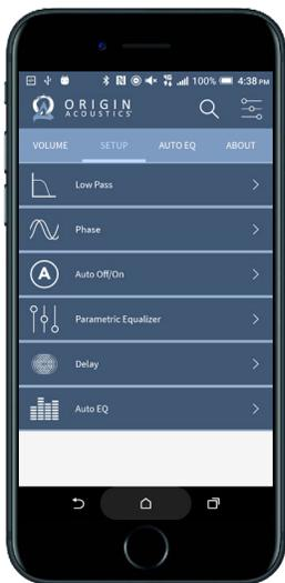
The proprietary Deep™ Sub phone app is available for iOS® and Android® operating systems. Here you can see the various parameters that can be adjusted. Included are Volume Level, Low Pass, Phase, Auto off/on, EQ and Delay.
