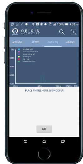
The Auto EQ option allows for the phone's microphone to be used to analyze the sub's output in the room and automatically adjust for the desired seating position.
