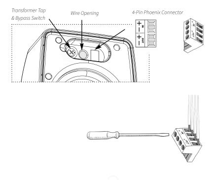
**7c.** When using multiple speakers you can connect the speakers either in parallel or in the loop through method as shown below.
