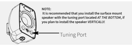
**1.** Run the speaker wires from the amplifier to the speaker location. Be sure to leave enough wire at the speaker location to feed through the hole in the speaker enclosure and wire to the terminal connector on the front.
