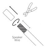
**7b.** Insert the wire into the correct square opening on the phoenix connector. Use a small flat head screwdriver to tighten the corresponding screw to secure the wire.
