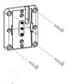
**3.** If the installation requires that the speakers be mounted on poles, you can attach the bracket to poles using U-bolt (not included).
