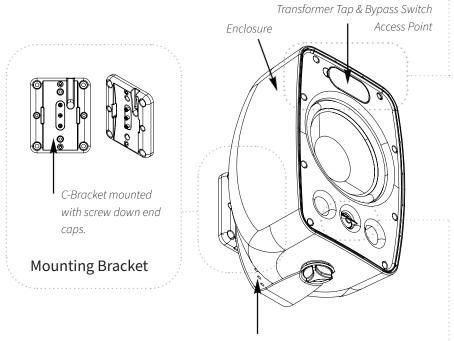
Weather Resistant POM Plastic C-Bracket with vertical angle adjustments
