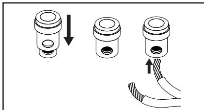
Figure 8.1: Connecting Wire
