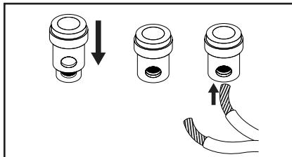
Figure 5.1: Connecting Wire
